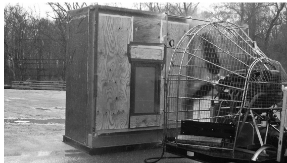
▲ Off-site mockup ("hot box") testing of window units provides controlled conditions for thorough evaluation.
