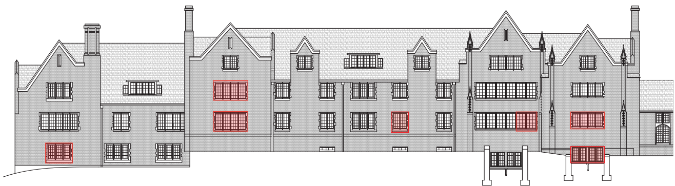
▲ Elevations can be keyed to the defect survey to identify levels of deterioration.
