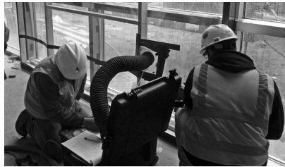
Window performance testing establishes thermal efficiency and moisture protection.
