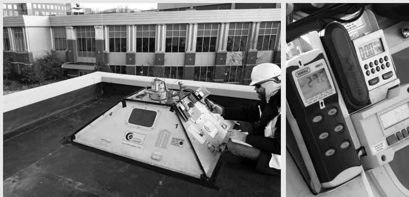
▲ Wind uplift testing for IEBC compliance and FM Global insurance certification.
