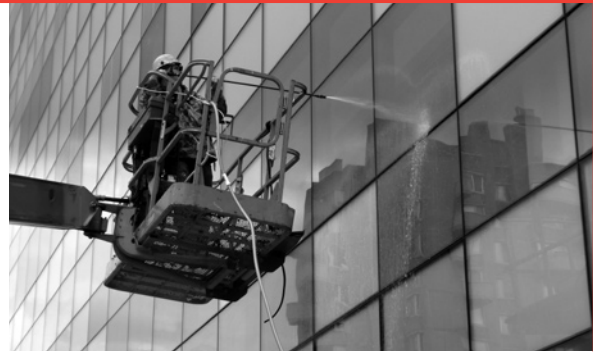
Commissioning often includes performance testing, such as water intrusion tests, to see that assemblies react as designed.
