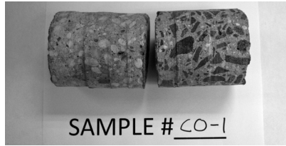
▲ Core samples of concrete may be tested for chloride content, strength, and composition to guide the design professional in evaluating the structure's resistance to corrosion.
