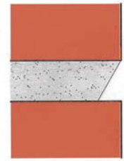
Struck (Not Acceptable)
