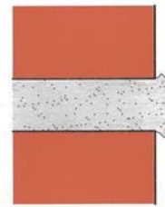
Extruded (Not Acceptable)
