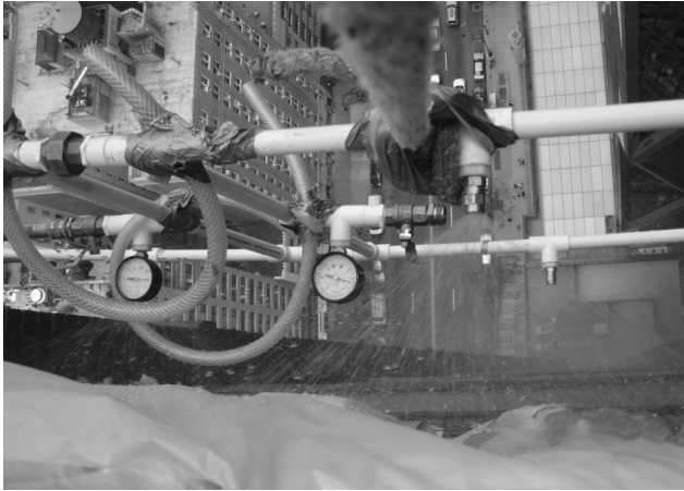
▲ High-rise buildings pose logistical challenges to water testing, including securing the test apparatus and managing overspray.
