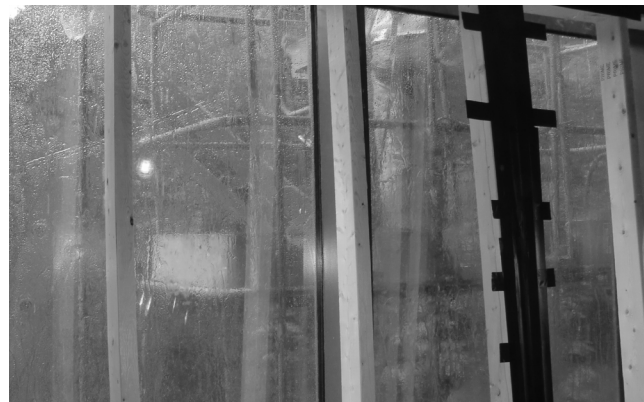
▲ Calibrated water penetration testing applies specific pressure differentials and flow rates in a controlled environment.
