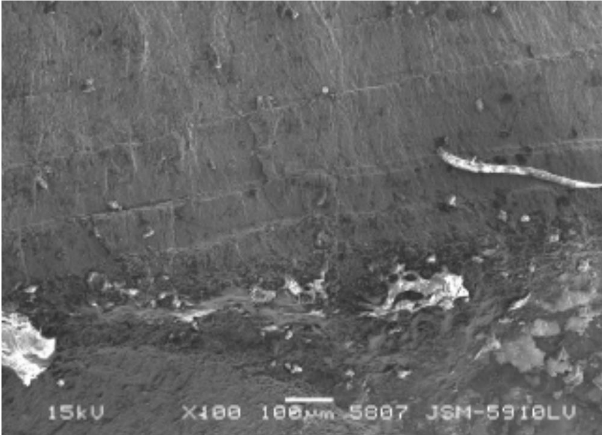
Photo 3 Scanning electron micrograph showing “beach marks” indicative of fatigue cycling.
