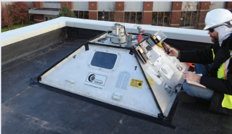
Wind uplift testing for IEBC compliance and FM Global insurance certification.
