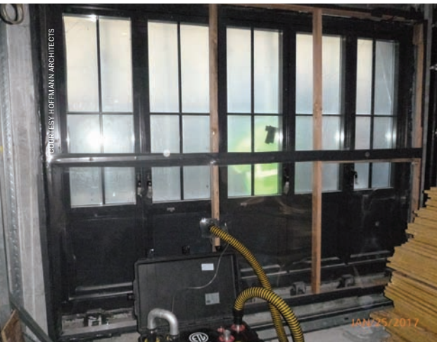
↑ Field tests confirm the storefront meets performance standards.
